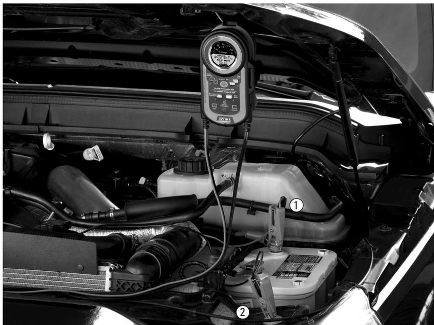
*Pictured: Typical DC charging clamp connections for a precharge status (with engine off), charging or just maintaining a fully charged battery with the DC charging clamps in a vehicle.*
