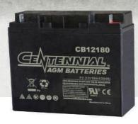
The series is a general purpose battery with 6~8 years design life in float service. It meets with IEC, JIS, BS and YDT standards. With advanced AGM valve regulated technology and high purity raw material, the series battery maintains high consistency for better performance and reliable standby service life. It is suitable for UPS/EPS, Telecom, power grid, medical equipment, emergency light and security system applications.
